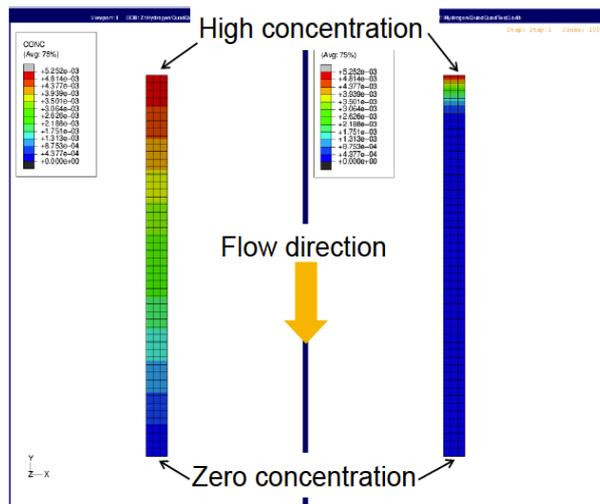
2D simulation of H diffusion in the presence (right) and in absence (left) of traps using ABAQUS.
