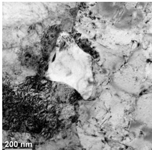
**TEM image of a TiC particle in one of the "TKSE-concept" model steels.**
