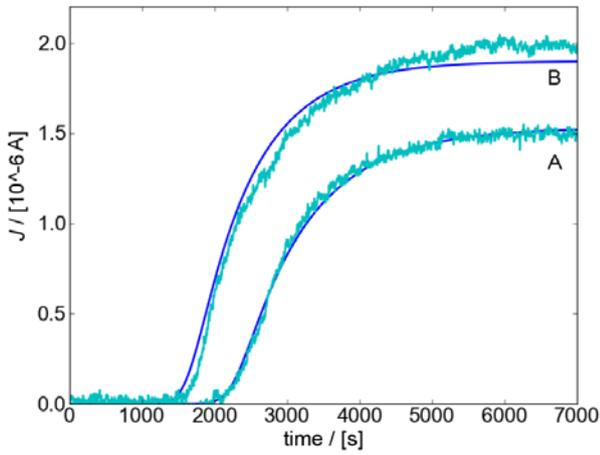
1<sup>st</sup> (A) and 2<sup>nd</sup> (B) permeation curves for one of our model steels fitted with FE-model.
